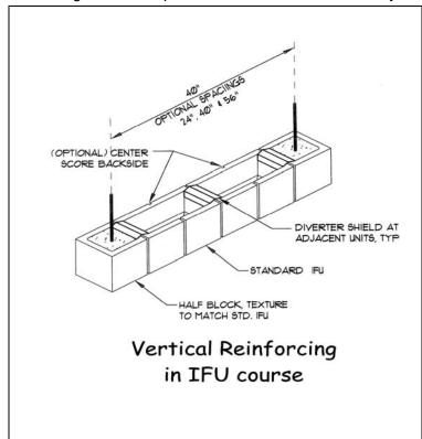
Structural continuity of CMU walls is maintained by the IFS. Conventional through wall flashing, to function properly, must completely penetrate both inside and outside face shells. This reduces the bond between adjacent masonry units. The IFU is placed in the wall using face shell bonding as with any typical CMU. Flexural strength of the wall is not compromised with the Integral Flashing System.
