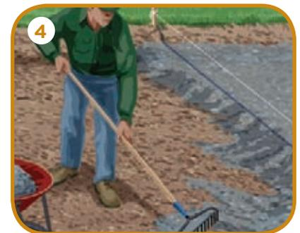
Spread aggregate base uniformly throughout the entire excavated area and 8 in. beyond perimeter lines. Base aggregate material should be processed 3/4" minus gravel or crushed concrete blend.
