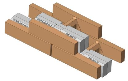
Walls built of Spec-Brik Hi-R H make a fully grouted barrier wall. The large open space behind the insert facilitates efficient placement of reinforcement and grout. Conduit for electrical needs is positioned within the core area just like a typical block wall.
