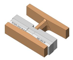
The web of Spec-Brik Hi-R H exceeds the minimum web, as well as all other ASTM C90 requirements. Insulation inserts are placed in the cmu at the factory. High-density EPS insulation is inserted into the notch molded into the web. The EPS insulation inserts are longer and taller than the block so when the mason builds the wall, insulation covers both the vertical and horizontal mortar joints.
